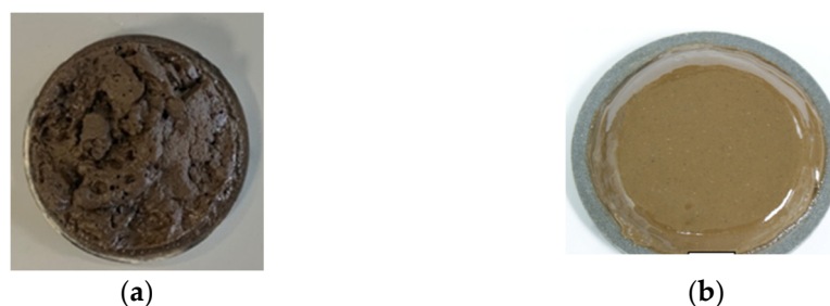
Figure 1. Images of drill-in fluids formulated from (a) synthetic-based mud, and (b) oil-based mud.
