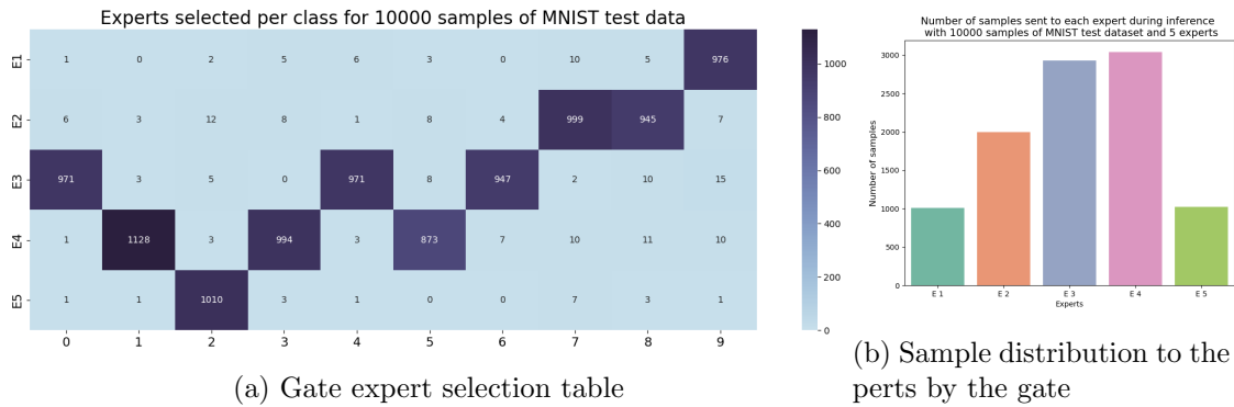
Figure B.2: Gate expert selection table of the reverse distilled gated MoE model trained in Step 2 of the peaking expert method from the pre-trained experts in Step 1, shown in Figure 6.4a for MNIST dataset. Gate is trained using stochastic model.
