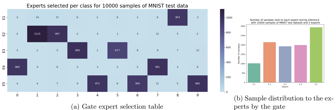
Figure 9.2: Gate expert selection table of the best performing model with L_s with 5 experts, which is the distilled MoE with output mixture model trained with L_s for MNIST test dataset.
