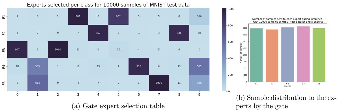
Figure 9.1: Gate expert selection table of the best performing model with L_{importance} with 5 experts, which is the top-2 model trained with L_{importance} for MNIST test dataset.
