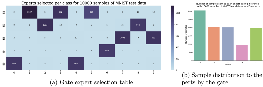
Figure B.4: Gate expert selection table of the reverse distilled gated MoE model trained in Step 2 of the peeking expert method from the pre-trained experts in Step 1, shown in Figure 6.4a for MNIST dataset. Gate is trained using output top-2 model.
