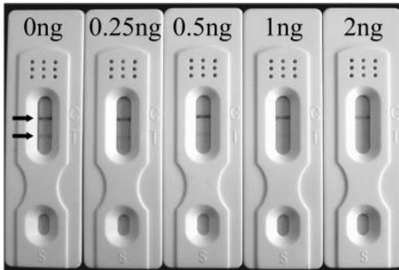
Figure 1.6: Detection results of the lateral flow assay method, with lead concentrations between 0 ng (0 ppb) and 2 ng, per ml (2 ppb) of water [92].
