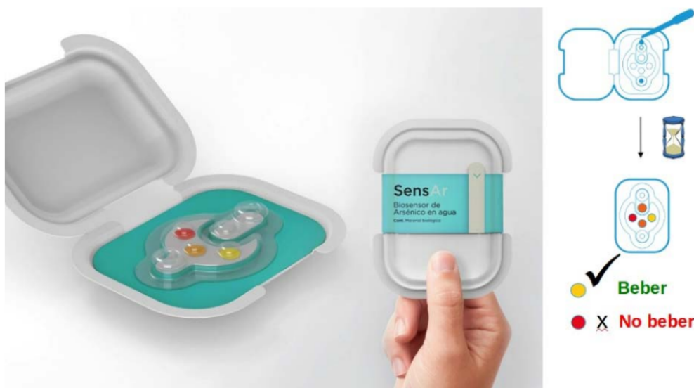
Figure 5.2: SensAr prototype, showing the casing and the biosensor colour results based on arsenic concentration [189]. If the biosensor presents a yellow colour, the water has an arsenic concentration below the WHO's limit. If the colour is orange then the sample has an arsenic concentration equal to WHO's limit, and if the colour is red then the concentration is greater than WHO's limit and the water should not be consumed, as shown in the Figure.
