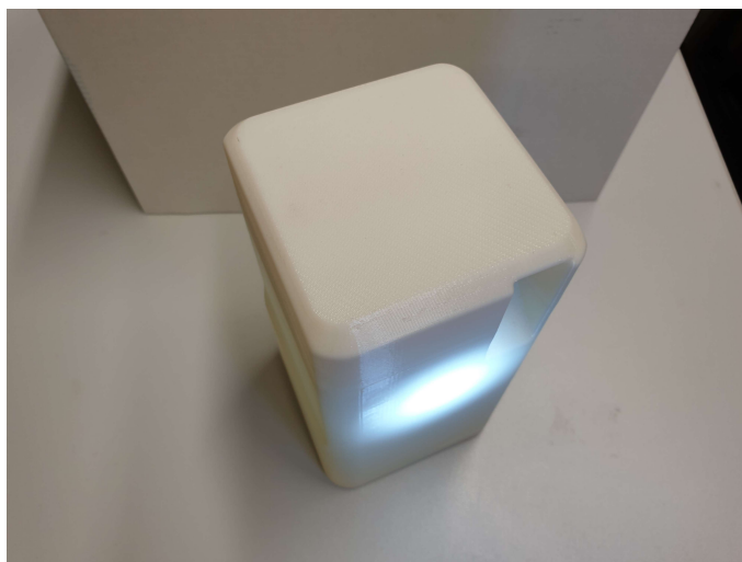
Figure 6.10: Example of data acquisition set up for light leak study. A torch was pointed at the PlomBOX from different directions
