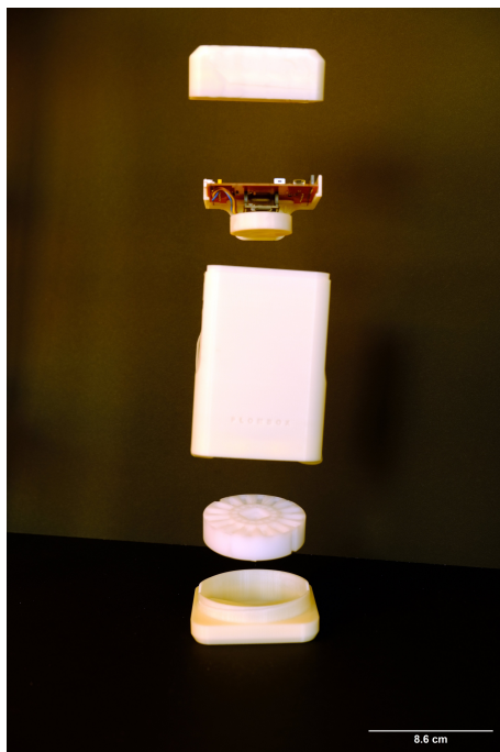
Figure 5.10: Photo of the PlomBOX's final design, with PCB visible at the top. [199]
