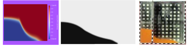
FIG. 3: Model validation using cwc simulation experiments at 0.2 sec time for the present study (left), Yeoh and Barber 25 (center), and Cruchaga et al 24 (right).
