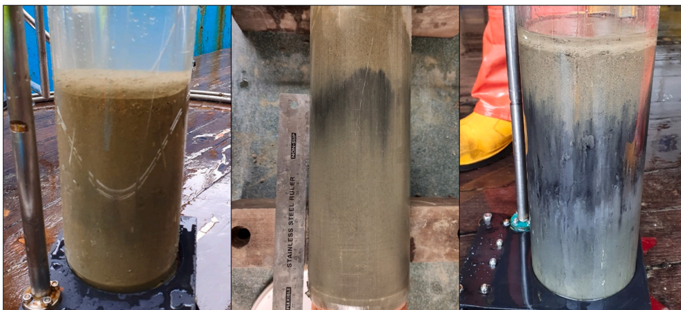
Fig. 3. Sediment core samples from BPM taken at 3200 m (left), 400 m (middle), and 100 m (right). A distinct layer of emerging black hydrocarbon contamination as well as newly deposited sediment can be seen in cores taken at proximity (400 m and 100 m).
