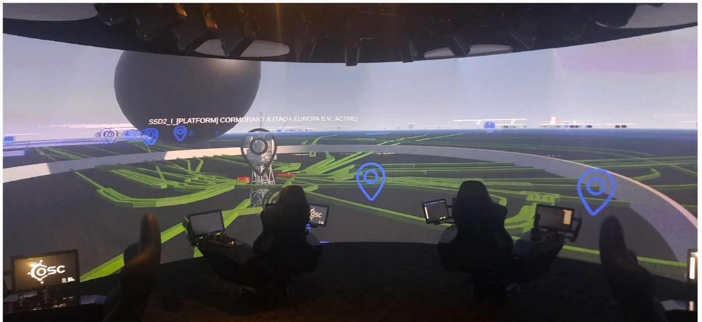
Fig. 10. View of the marine simulator dome showing the area around Cormorant A. Grey circle shown is the safety zone around Cormorant A, green lines are pipelines, red lines are freespans, black pin marks the platform, and blue pins mark subsurface infrastructure. The large black sphere represents CO 2 emissions for Cormorant A in 2020 (37,874.51 tonnes). (For interpretation of the references to colour in this figure legend, the reader is referred to the Web version of this article.)
