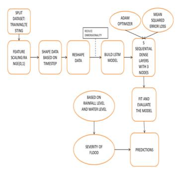
Fig:3 Overall Workflow for Flood Prediction
