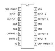
Fig.4 Pin description of dual L293D H-Bridge motor
