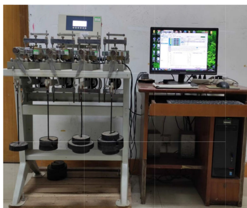
FIGURE 6: The direct shear experiment of tailing sands sample.
