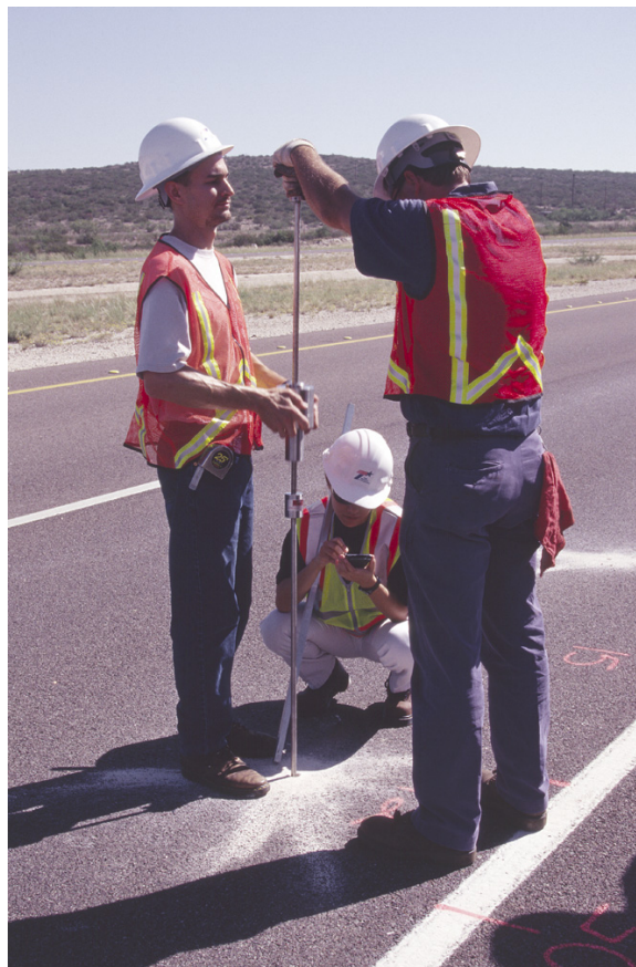
Figure 4. TxDOT staff conducting DCP test at SRBA site on I-10 in Pecos County, Texas.
