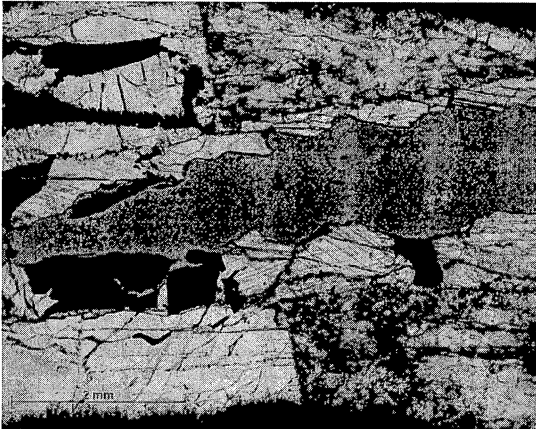
Figure 9. Fractured carbonate/pyrite concretions with multiple phases of fracture sealing cement, Hardie Unit #1 core. Samples from (a) 7,803 ft and (b) 7,817.5 ft. (c) Plane light photomicrograph of anhydrite, calcite and pyrite cements in the fracture in (a). These are similar to the fractures in the Paxton Isaac well concretions.
