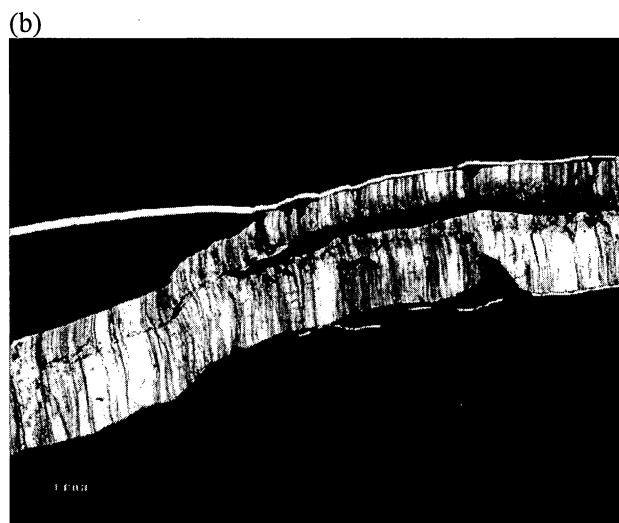
Figure 13. (a) Low-angle fractures in the Hardie Unit #1 core, 7,889.5 ft. (b) morphologies of these fractures can be irregular, with fracture walls being non-planar.
