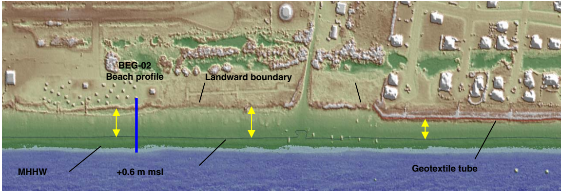
Figure 8. Lidar topographic relief image of Galveston Island State Park and Pirates Beach subdivision. Note difference in beach width between the natural beach and in front of the subdivision.
