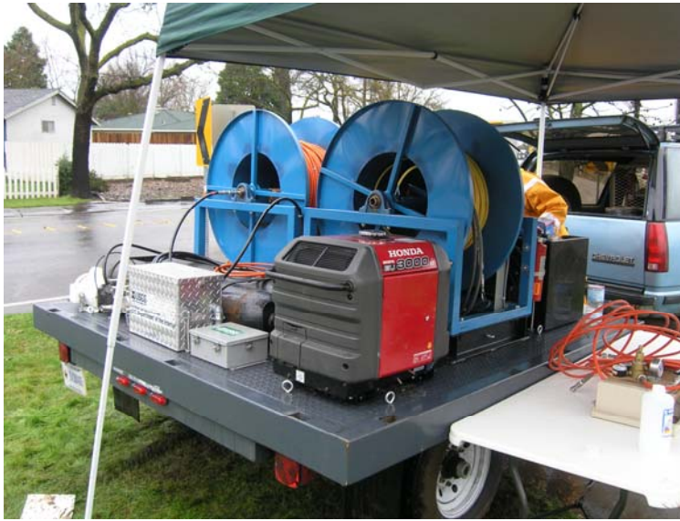
Figure 25. View of sampling system for well bore flow and depth-dependent sampler used in field studies. There are two Bennet pump reels with hoses: one for dye injection and the other for sample collection. A generator is required for the pump. All equipment is mounted on a flat trailer.
