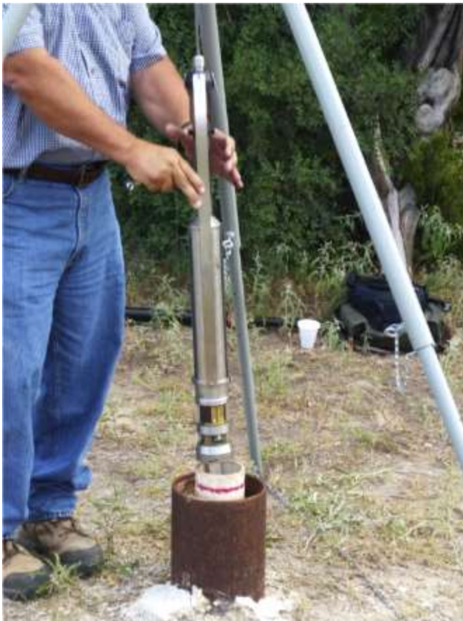
Figure 10. Video camera being inserted in water well (Barnett Shale area)
