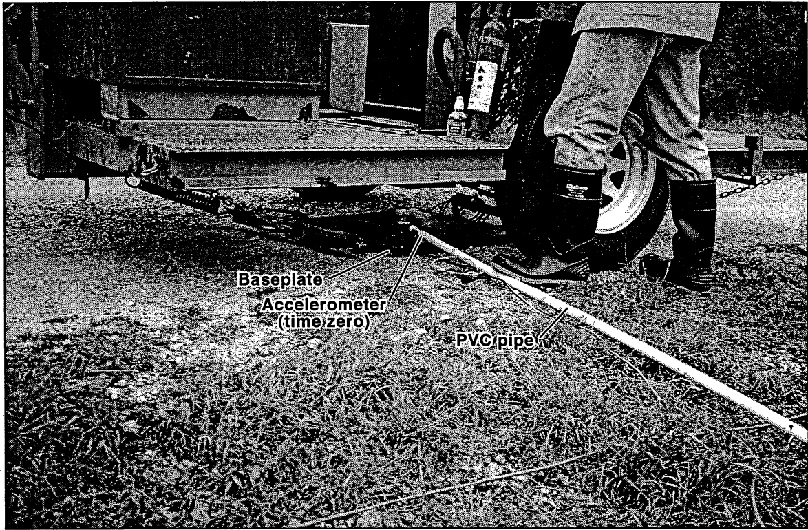
Fig. 16. Baseplate of weight-drop source and accelerometer used to establish time zero of the seismic impulse.
