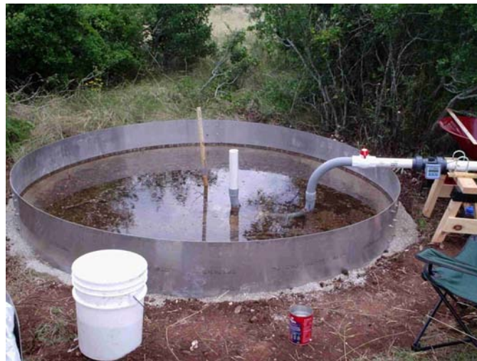
Figure 2. Ring infiltrometer ponding water on a sinkhole with flow meter and control section.
