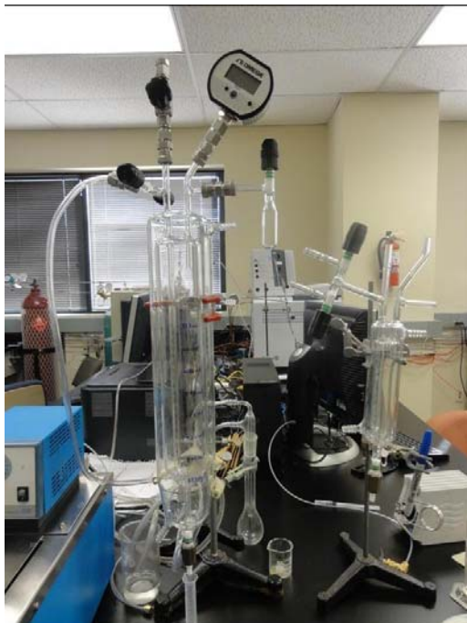
Figure 4. Picture of degassing glass apparatus in BEG gas geochemistry laboratory
