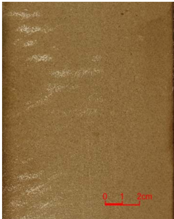
Fig. 2A Uniform fine-grained sandstone at 9128 ft, Well OCS-G-3733 A-6, Matagorda Island.
