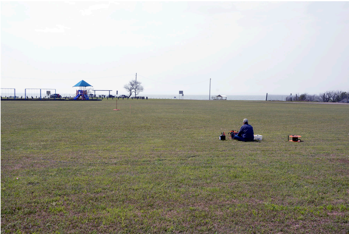
Figure 8. Bureau staff acquiring time-domain EM data near Olivia in the Olivia quadrangle, March 2020.
