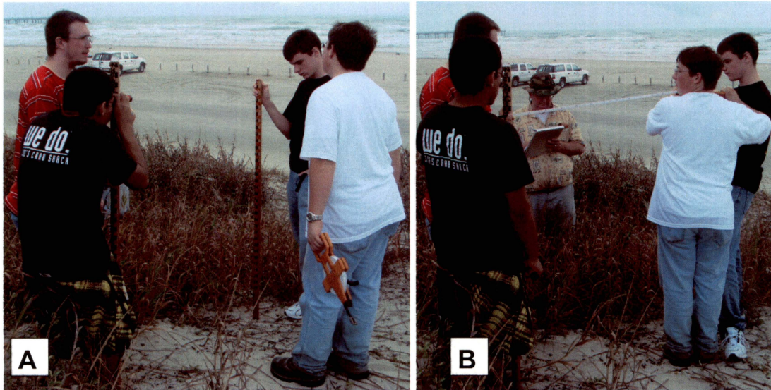
Figure 2. Students using (A) a sighting level to determine vertical offset between Emery rods and (B) a metric tape to measure horizontal distance.
