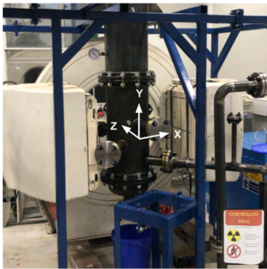
Fig. 2. The Forte can accommodate large experiments for investigation with PEPT due to its dual-headed geometry. The coordinate system in this work begins in the center of the FOV.
