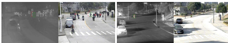
Fig. 4. Example images from the VOT-RGBT2020 dataset. The left two frames illustrate the synchronization issue in the RGBT234 dataset [43] and the right two frames the small object issue.
