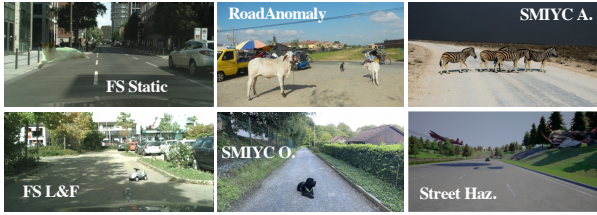
Figure 2: Samples from previous OOD datasets to visually support Tab. 1: FS Static has unrealistic OOD objects while RoadAnomaly and SMIYC datasets have strong domain shifts from Cityscapes. FS L&F (which manually inserts OOD objects) and StreetHazards (full simulation) have large set-up costs.
