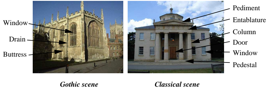
Figure 3: Example of some primitives used to construct Gothic and Classical architecture.
