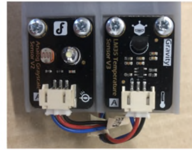
c grayscale and temperature sensor left: DFRobot Gravity Grayscale sensor (analog) right: DFRobot Gravity LM35 Temperature Sensor (analog)
