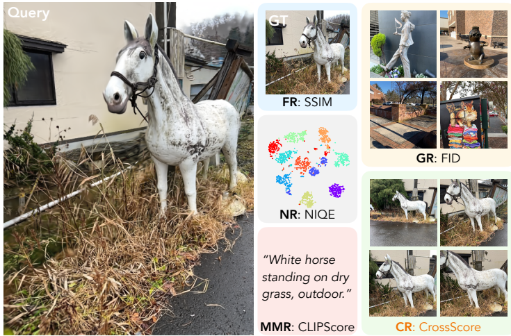
Fig. 1: We propose a novel cross-reference (CR) image quality assessment (IQA) scheme, which evaluates a query image using multiple unregistered reference images that are captured from different viewpoints. This approach sets a new research trajectory apart from conventional IQA schemes such as full-reference (FR), general-reference (GR), no-reference (NR), and multi-modal-reference (MMR).
