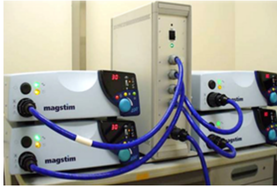
Figure 1.10: Quadripulse stimulation setup. Four Magstim 200 2 stimulators are connected to combine the output through one stimulation coil with a specially designed combining module. Reproduced from (Matsumoto et al. 2020)
