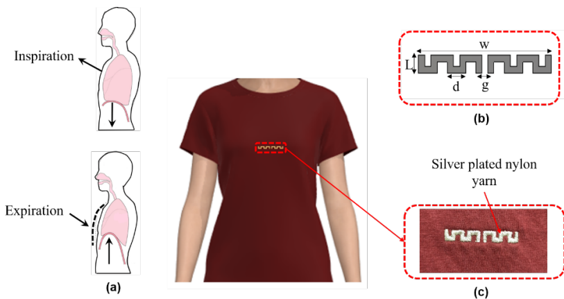
Figure 4.13: (a) Simplified illustration of the lungs during inspiration and expiration, (b) Geometry of the proposed antenna sensor, (c) Embroidered prototype.
