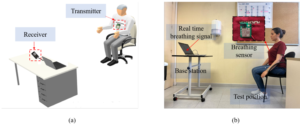
Figure 4.23: Person under test wearing the e-textile for breathing monitoring: (a) experimental setup configuration and (b) photograph of the experimental setup.
