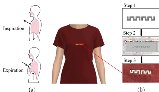
Fig. 1. (a) Simplified illustration of the lungs during inspiration and expiration, (b) Fabrication process of the embroidered antenna-sensor integrated into a cotton T-Shirt.
