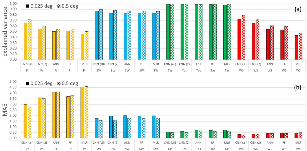
Figure 3. Comparison among ML algorithms (CNN, convolutional neural network; RF, random forest, ANN, artificial neural network and MLR, multiple linear regression) applied to the study domain for the test period 2005–2014: explained variance (a); mean absolute error (MAE) Pr: mm/day, Tas: °C, SW: MJ/m2/day, WS: m/s (b). CNN(all) included all predictors, and CNN(2) included only two predictors (i.e., JRA55 SLP and the corresponding JRA55 variable to be downscaled). The downscaled outputs are presented at two resolutions (0.5° and 0.025°). Pr, precipitation; SSR, surface solar radiation; Tas, air temperature; WS, wind speed. See also Table S3.
