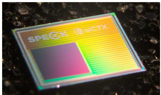
Fig. 1. Photograph of the realised "Speck1" ASIC. The rectangle at the bottom left of the chip is the 128x128 pixel event sensor for machine vision applications, while the rest of the area is occupied by the processing cores and the NoC.
