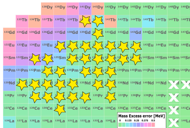
Fig. 3. Mapping the mass surface for the neutron-deficient lanthanides with the FRS Ion Catcher while employing mean range bunching. The figure shows a section of the chart of the nuclides in the range from La to Dy. Stable nuclides are marked with a white X. The 37 nuclides, which were measured in a single setting of the FRS and in a single setting of the MR-TOF-MS are marked by stars.
