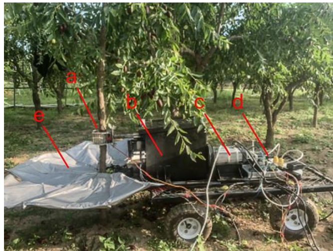
Figure 4. Vibration test of jujube trees, where a is the clamping mechanism; b is the excitation mechanism; c is the frequency modulation motor; d is the walking mechanism; e is the fruit collection mechanism.
