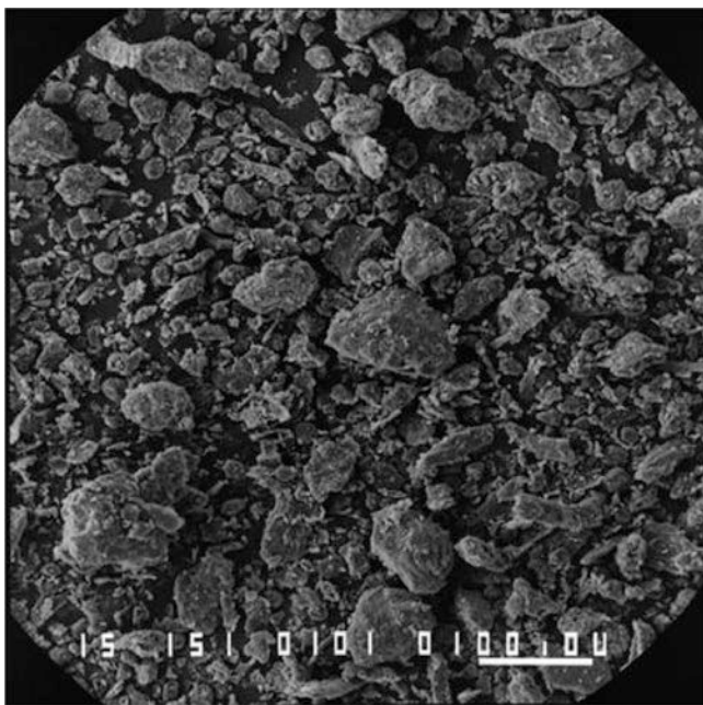
Fig. 12.3 Particle size variation in the manually (in a mortar with a pestle) crushed Nifedipine tablet (Adalat® 10 mg retard). Scale bar in SEM is 100 \mu\text{m} [27].
