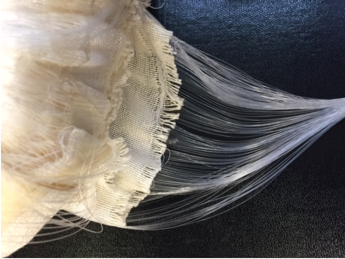
Fig 12: POFs woven via the weft and bundled together to connect to the light source.
