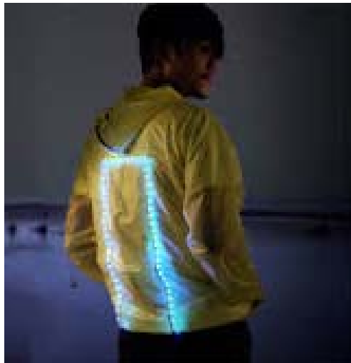
Fig.2: LED yarn developed by PEGA Design and Engineering.
