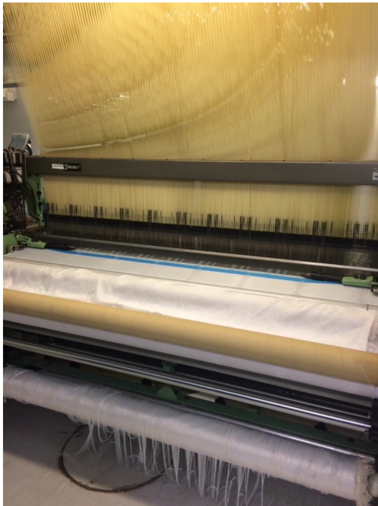
Fig. 9: Dornier Weaving Loom PTV 8/J with the STAUBLI Jacquard Head JC6.
