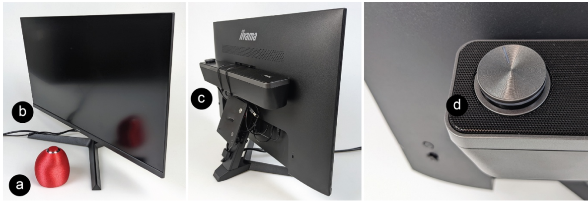
Figure 11: During the pilot study, the Switch2Move home system consisted of a tangible controller (a) connected to a 27-inch external monitor (b); a media player attached to the backside of the monitor (c), and a speaker with a volume control knob (d).
