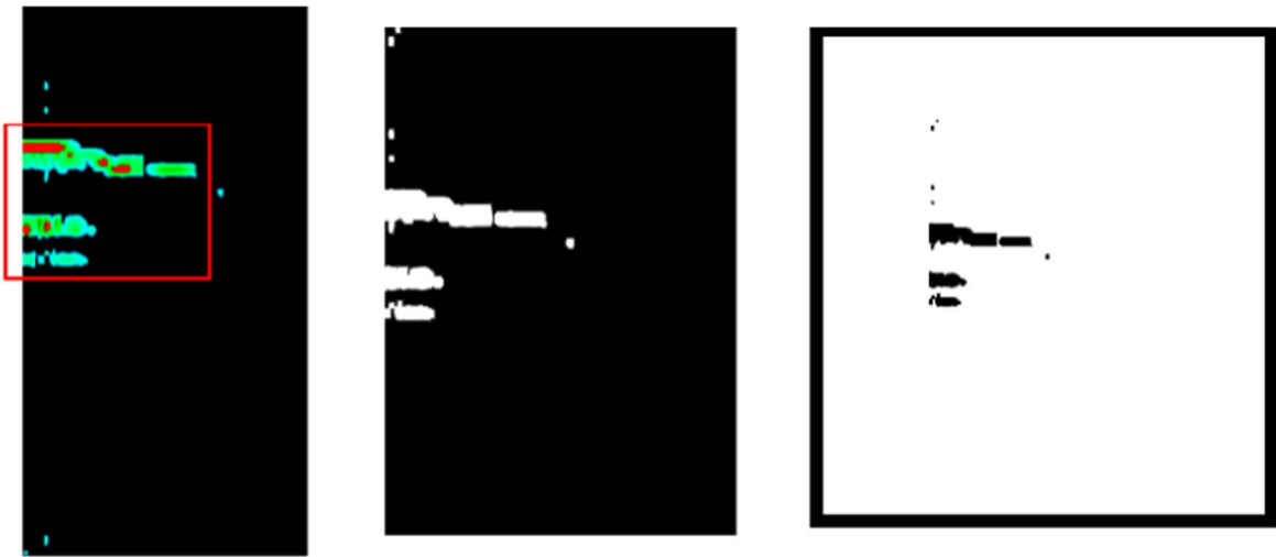
Figure 6. Full processing, original cropped ionogram (left) with binary mode (middle), and resized image using ESA 800 \times 600 px standard (right). As it can be seen in the binary mode image, the loose pixels have been removed, producing shapes without gaps. In the image, in a red box, the red areas that disappear with the OpenCV operation have been marked. It is done to avoid detecting several objects through those “holes.”
