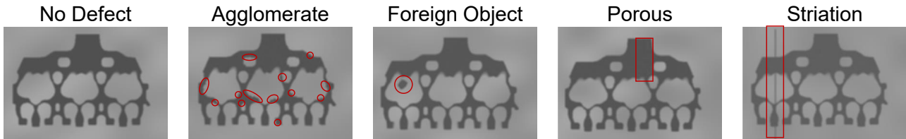
Figure 7: Anomaly types included in the synthetic data (red: highlighted location of anomaly). Agglomerate: accumulation of unwanted loose components into a solid compound. Foreign object: unknown objects on the printbed. Porous: temperature difference in the direction of print head movement. Striation: vertical striations from excess binder, sand or nozzle-clogging.
