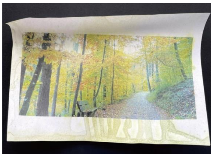
Figure 4.2.12: Preprinted cellulosic paper treated with wet-chemical method showing deformation and wrinkling of the paper and damage of the printed content due to ink diffusion. Reprinted with permission from [25].
