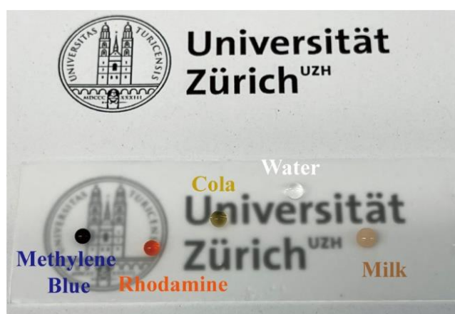
Figure 4.3.11: Aqueous droplets (10 \mu\text{L} ) of water, rhodamine, methylene blue, milk, and cola on the surface of 6-seg-ETCS-SC-SNRs modified sample. Adapted with permission from [23].
