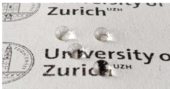
Figure 4.2.9: Pictures showing water droplets (10 \mu\text{L} ) spherically contact with the printed SNRs-A4-paper. Reprinted with permission from[25].
