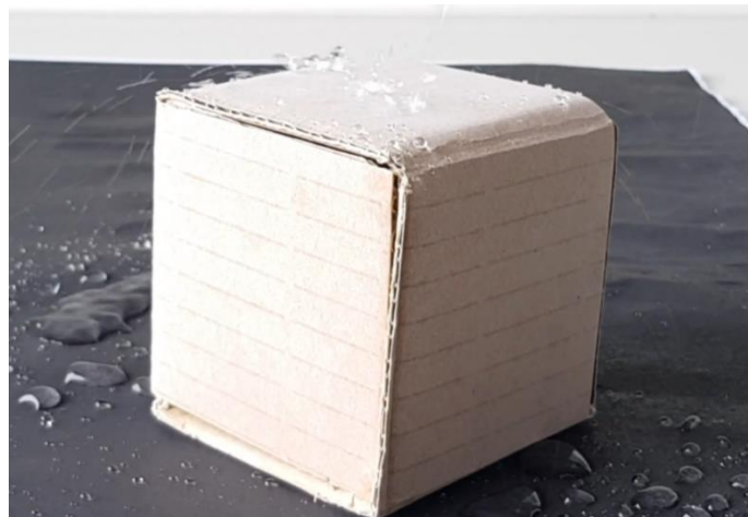
Figure 4.2.15: Water jet bounces off the package box decorated with ETCS-SC-SNRs.
