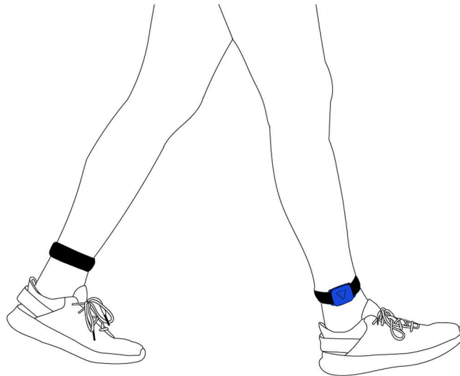
Figure 1. Positions of the sensors attached laterally above the ankles.
