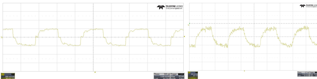
Figure 11.8: Clock signal measured at the connector of the FPGA (left) and the connector of the quad module to the TEPX half-disk (right).
