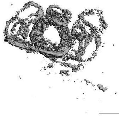
**Figure 9.** Reconstruction of  $\mu$ -CT data of explanted tissue with residual magnesium scaffolds six months following implantation. Bar indicates 5 mm.
