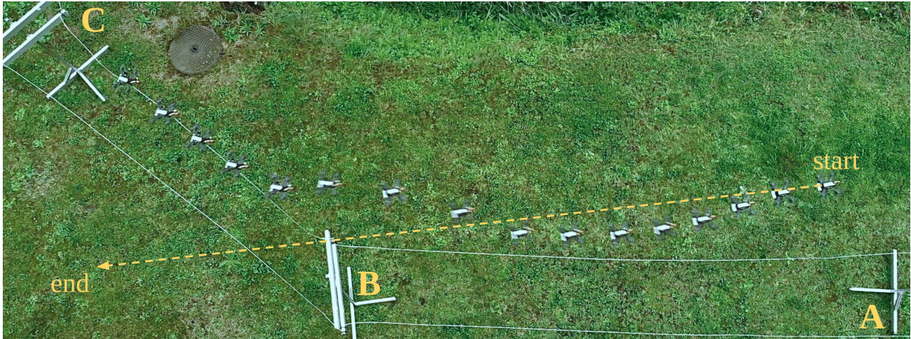
Fig. 1: A quadrotor performing power line inspection in a power line test environment with three masts (labelled: A, B, and C) using our proposed approach. The original rough reference trajectory is depicted in yellow and the drone deviates from it while avoiding obstacles (the power masts) and keeping the power line visible in the field of view of the onboard camera.
