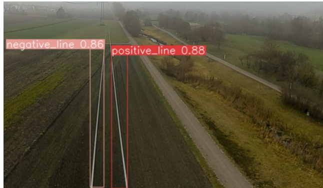
Fig. 6: A sample result of our line detector validated using a real-world image. Our detector shows correct prediction with high confidence in a challenging real-world scene, despite only being trained with synthesized images.
