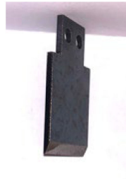
Figure 3. Specially made tip for Universal Testing Machine.
