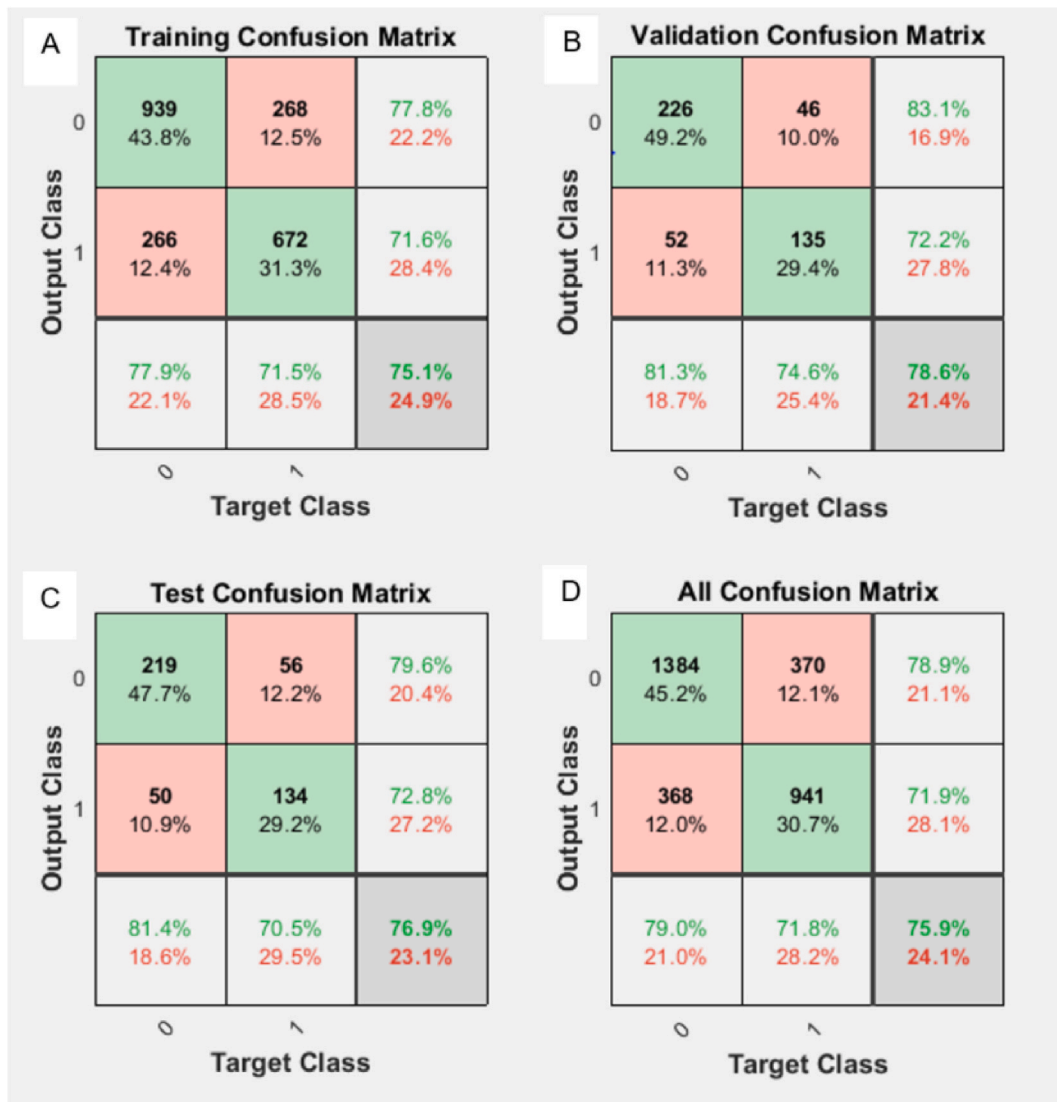
Fig. 5. Highlights confusion matrices with a coincidence rate ( \pi ) of more than 75% for each sample and a total coincidence rate of 75.9%. The ROC curve of the BPNN model is demonstrated in Fig. 6. The total AUC added up to 0.827 and is another indication of the high level of discrimination.
