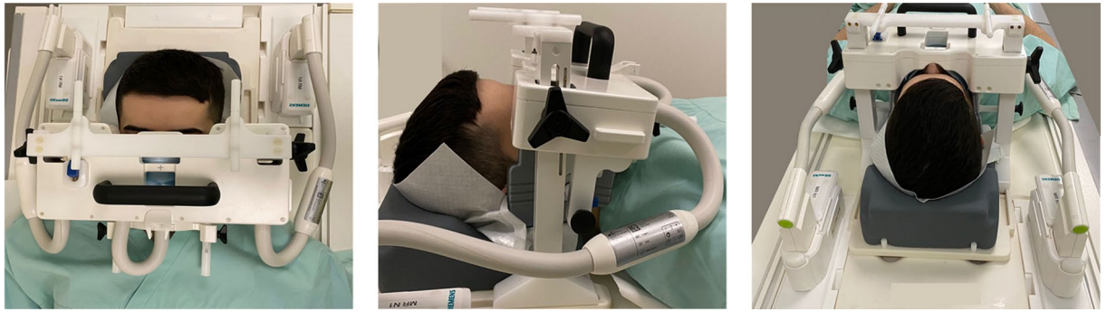
Figure 1. All study participants underwent 3 Tesla MRI (Skyra, release VE11e, Siemens Healthineers, Erlangen, Germany) using a dedicated 15-channels mandibular coil (NORAS MRI products, Hoechst, Germany). The mandibular coil used in this study has a field of view of 32 \times 16 \times 16 \text{ cm}^3 and is an optimized 14+ 1 receiver coil array and positioning system specifically designed for high-resolution imaging of dental structures in the oral cavity.
