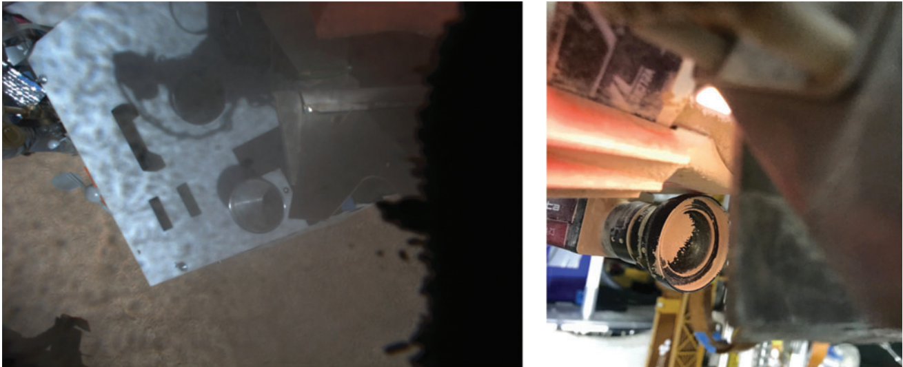
FIG. 7. (Left) arm camera image acquired to determine whether sample is in the scoop. The image is obscured by dust on the lens. (Right) Photograph of arm camera lens collected after a drilling operation showing dust accumulated on the lens.
