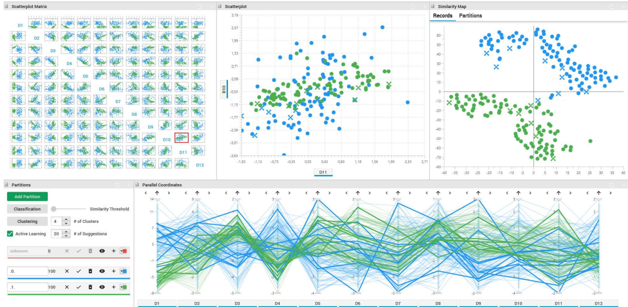
Fig. 1: The mVis tool (Chegini et al., 2019a), showing the SPLOM at top left, detailed scatterplot top middle, similarity map top right, and parallel coordinates bottom right, for the MNIST2 dataset. The partitions panel at bottom left shows the currently defined classes (label alphabet). Instances are colour-coded by class, here green for 1s and blue for 0s. Instances with confirmed labels are shown as crosses in the scatterplots and similarity map and as thick lines in the parallel coordinates. Suggestions from the classifier are shown as solid circles in the scatterplots and similarity map and as thin lines in the parallel coordinates.
