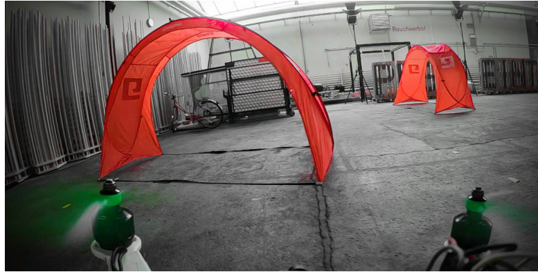
Figure 2.2 – Our quadrotor flies through an indoor track. Our approach uses optimal filtering to incorporate estimates from a deep perception system. It can race a new track after a single demonstration.
