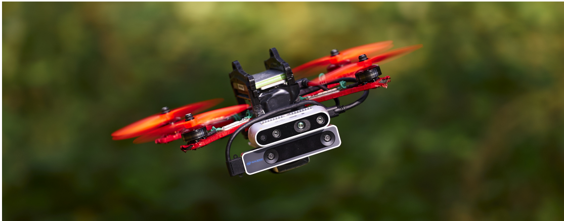
Figure 1.2 – A vision-based quadrotor developed in this work, navigating autonomously in the forest. The quadrotor can navigate towards given waypoints at speeds up to 40 \text{ km h}^{-1} , without the need to build an accurate 3D map of its surroundings. This capability is enabled by deploying a machine-learning approach directly on the quadrotor: a deep neural network is fed observations from an onboard camera, an estimate of the platform state, and a reference direction to compute a collision-free receding-horizon trajectory. Employing such a data-driven methodology allows to achieve a low-latency perception-action loop while maintaining robustness to sensor noise.
