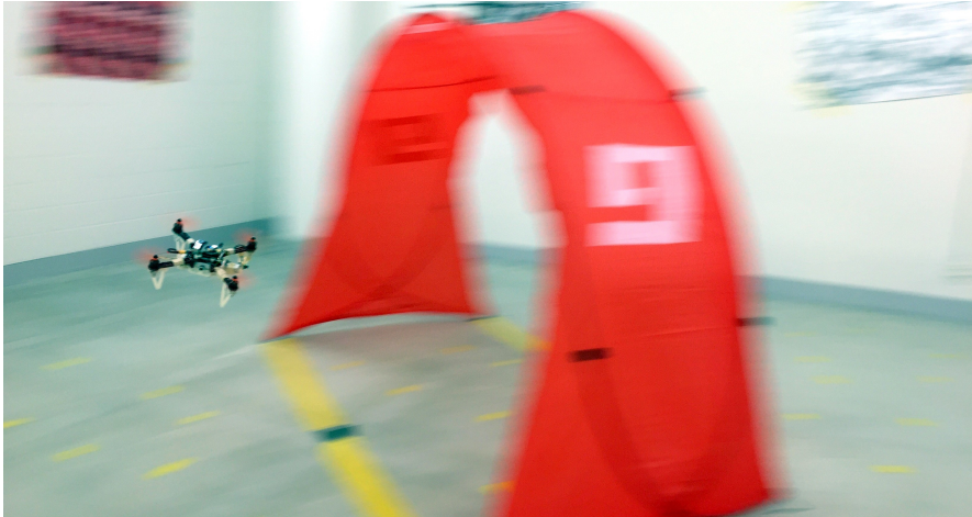
Figure 2.1 – By combining a convolutional neural network with state-of-the-art trajectory generation and control methods, our vision-based, autonomous quadrotor is able to successfully navigate a race track with moving gates with high agility.
