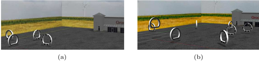
Figure D.4 – Illustration of the simulated tracks. The small track (a) consists of 4 gates and spans a total length of 43 meters. The large track (b) consists of 8 gates placed at different heights and spans a total length of 116 meters.
