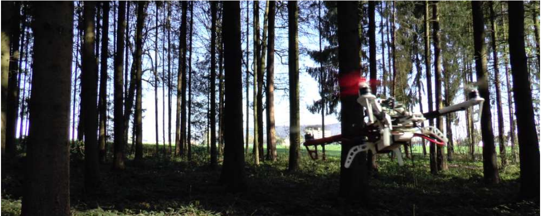
Figure 2.14 – Illustration of the quadrotor autonomously exploring a forest. The quadrotor reached speeds up to 2 \text{ m s}^{-1} .
