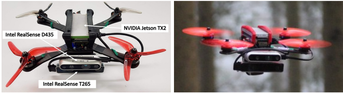
Figure F.8 – Illustration of our experimental platform. The main computational unit is an NVIDIA Jetson TX2, whose GPU is used for neural network inference and CPU for the control stack. Sensing is performed by an Intel Realsense T265 for state estimation and an Intel Realsense D435 for depth estimation.
