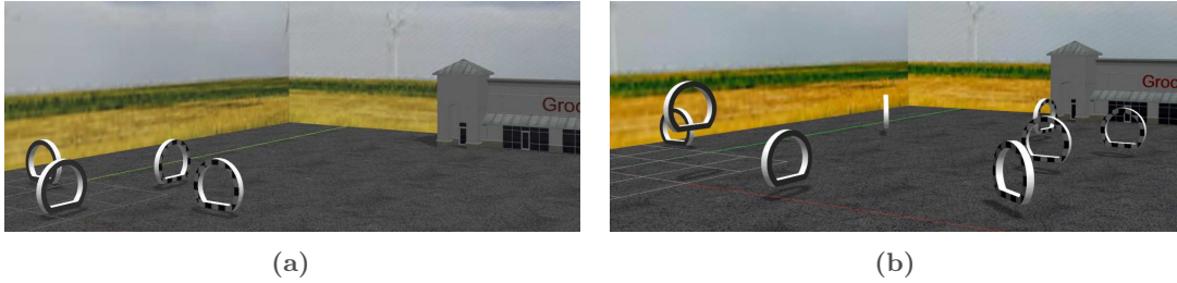
Figure A.3 – Illustration of the small (a) and large (b) simulated tracks. The small track consists of 4 gates placed in a planar configuration and spans a total length of 43 meters. The large track consists of 8 gates placed at different heights and spans a total length of 116 meters.
