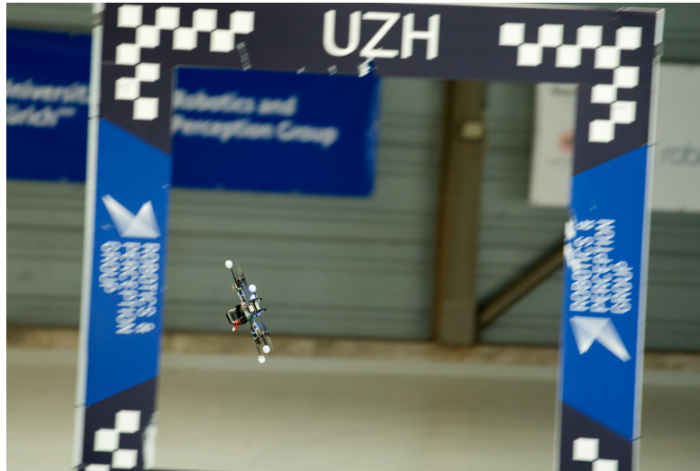
Figure 2.9 – In this work, I present a novel approach for autonomous drone racing that only relies on onboard sensory observations and onboard computation. The approach combines model-free reinforcement learning with residual models identified from real data to achieve champion-level performance on the task of vision-based drone racing.
