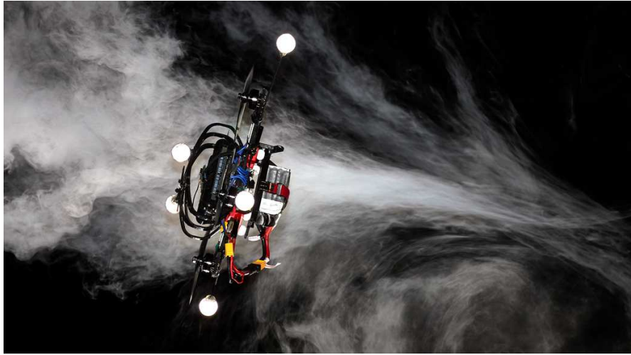
Figure 2.10 – Our quadrotor platform reaches its physical limits at a pitch angle of 80 degrees while performing a lemniscate trajectory in our experiments. Throughout the trajectory, the platform reaches speeds of up to 14\text{m s}^{-1} and accelerations beyond 4g .
