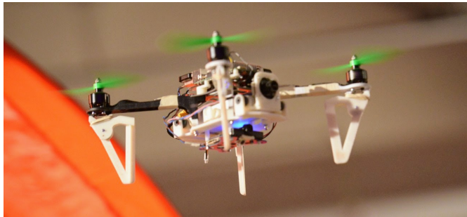
Figure B.4 – Our platform, equipped with an Intel UpBoard and a Qualcomm Snapdragon Flight.
