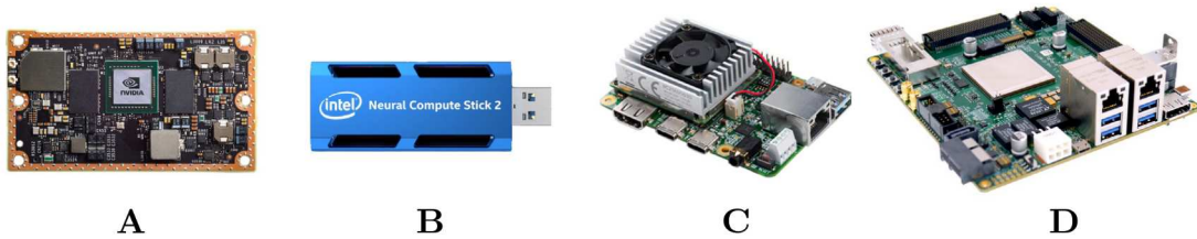
Figure 1.5 – Neural network-based approaches can be efficiently computed on specialized hardware such as graphics processing units (GPUs), tensor processing units (TPUs), or even field programmable gate arrays (FPGAs). Examples of such hardware accelerators include the NVIDIA Jetson TX2 (A), which contains a built-in GPU; the Intel Movidius Neural Compute Stick (B), which contains a specialized vision processing unit optimized for neural network inference; the Google Coral board (C), which contains an integrated TPU; and the TySOM development board (D) combining an FPGA with an ARM Cortex processor.
