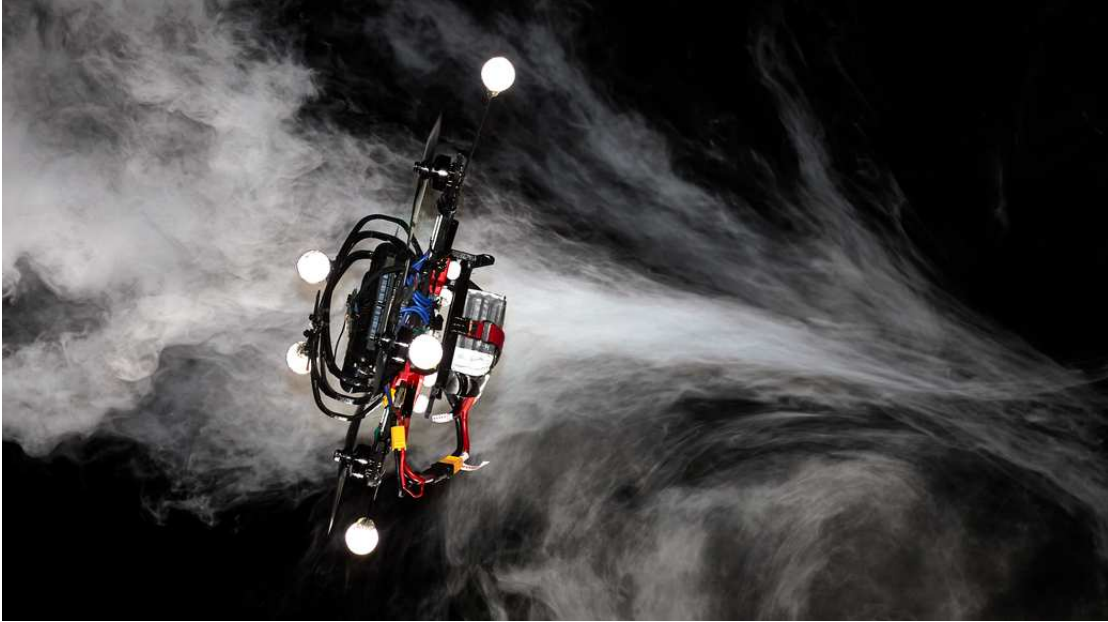
Figure I.1 – Our quadrotor platform reaches its physical limits at a pitch angle of 80 degrees while performing a lemniscate trajectory in our experiments. Throughout the trajectory, the platform reaches speeds of up to 14\text{m s}^{-1} and accelerations beyond 4g .
