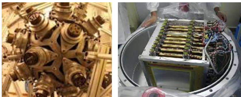
Fig. 4. Left panel the Total Absorption Calorimeter (TAC), Right panel Parallel Plate Avalanche Chamber PPAC.
