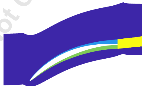
FIGURE 5: Example domain decomposition for the NACA65 Tu4 case.
