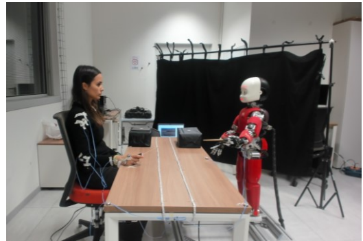
Figure 1. Experimental setup. A controlled and repeatable interactive setup was created. Both the participant and iCub are positioned in front of a rectangular-shaped table with two strips of LEDs. They both hold a wooden stick in order to hit the rubber pad to register their temporal estimate. Markers are attached to their arms to track their kinematics.
